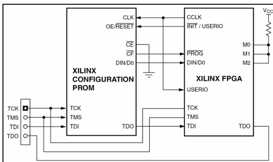
Figure 5.1 – Serial hardware interface
