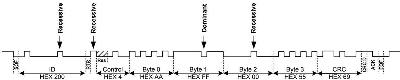
Figure 6.7 – Test Data packet for transmission via CAN.
