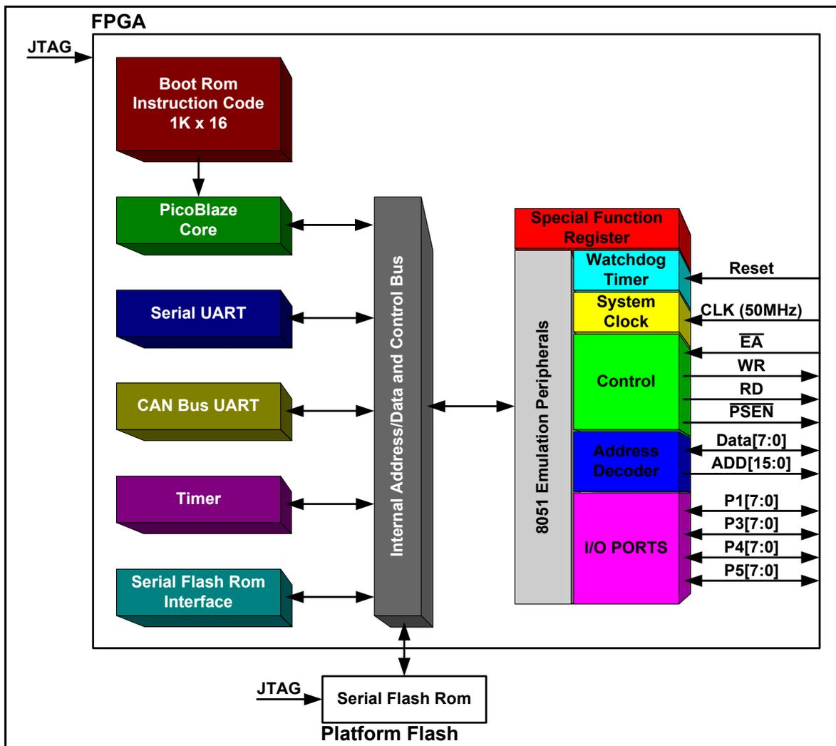
Figure 1.1 – Block diagram over BGEPB1 Emulated 8051 Microcontroller
