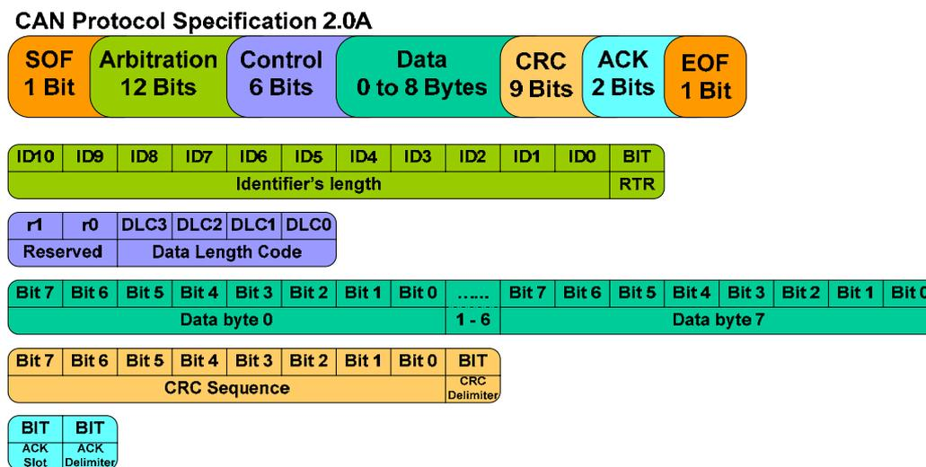
Figure 6.2 – CAN protocol Specification 2.0A
