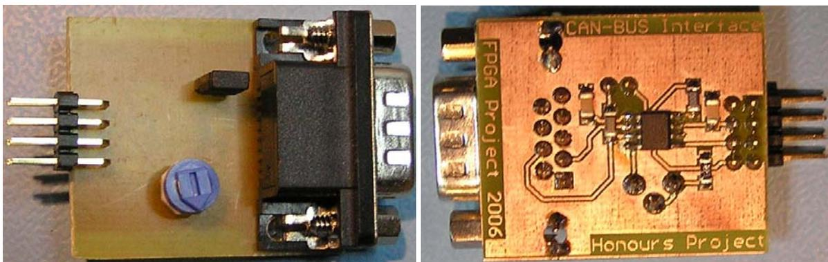
Figure 6.6 – Pictures of the CAN bus interface.
