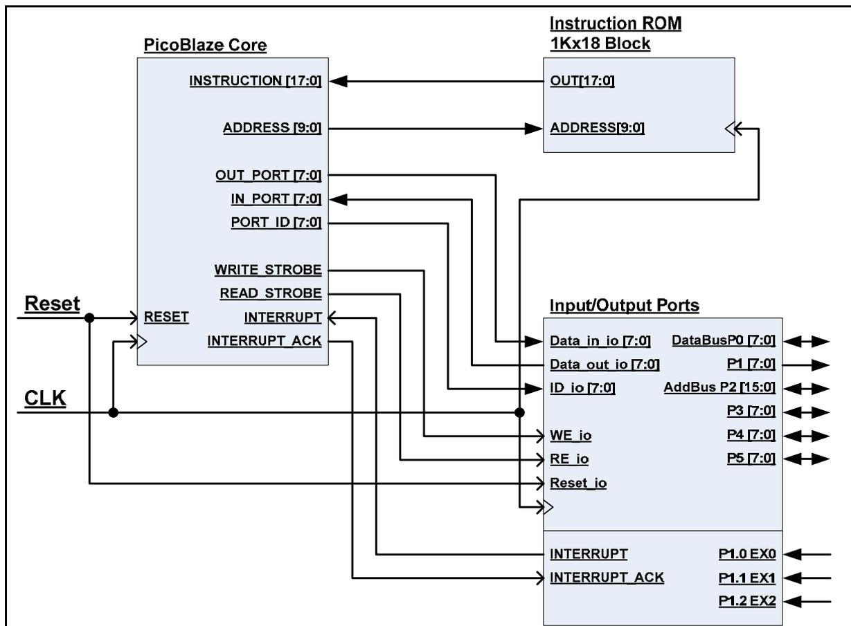
Figure 2.2 – Block diagram over I/O interface
