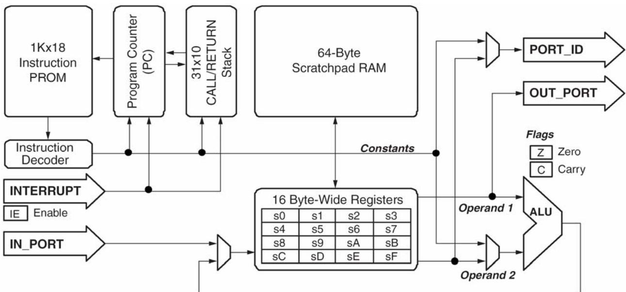
Figure 2.1 – PicoBlaze embedded microcontroller Block Diagram
