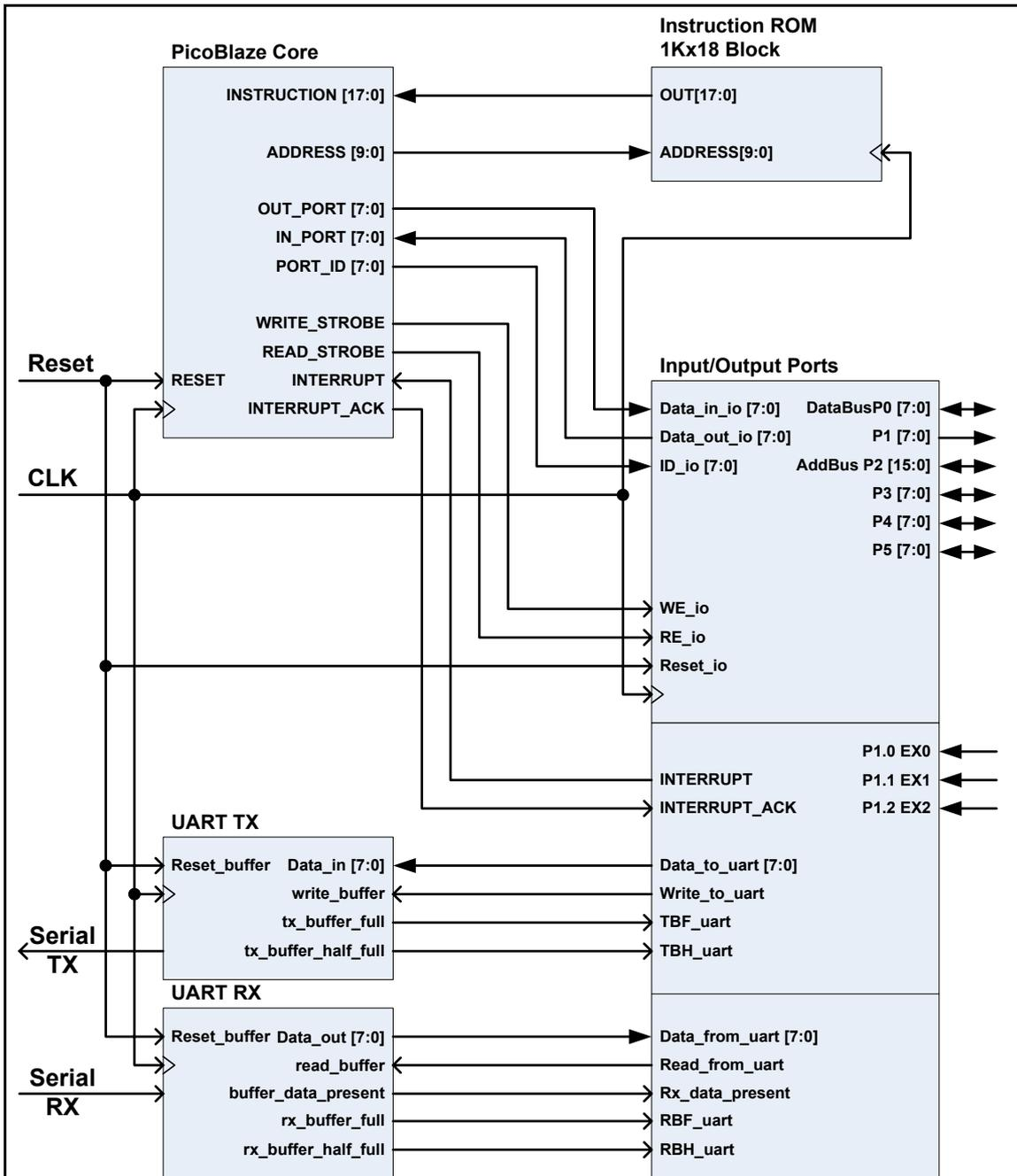
Figure 3.2 – Block diagram with TX and RX UART.
