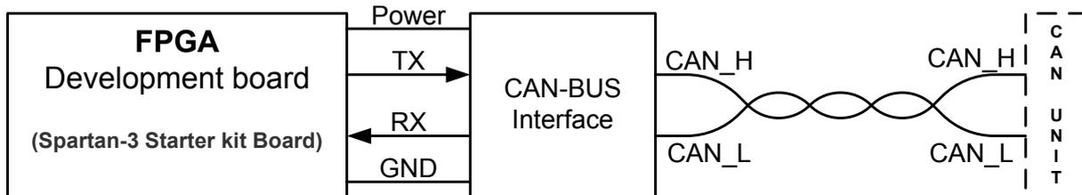
Figure 6.3 – Block diagram over CAN-BUS Interface.
