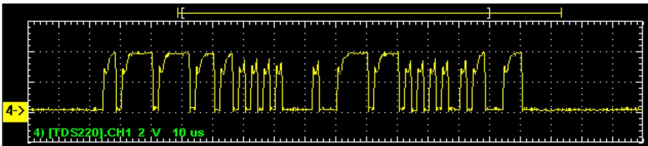
Figure 6.10 – Oscilloscope picture from transmission of CAN data packet.
