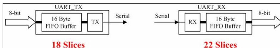
Figure 3.1 – Serial UART block diagrams.
